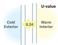
Because of the heat transfer driven by the buoyancy of warm air, overhead glazing exhibits a lower level of insulating performance (and therefore a higher u-value) than does glazing installed in a vertical wall, with everything else being equal.
