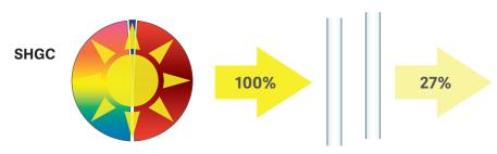
In most geographic locations, especially those in warm climates, a lower SHGC is desired to block heat and reduce the need for air conditioning. In colder climates, a high SHGC may be desired to take advantage of passive heat gain, lowering building heating costs.
