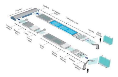
Figure 3 – Wet Coating Mirror Production Process
